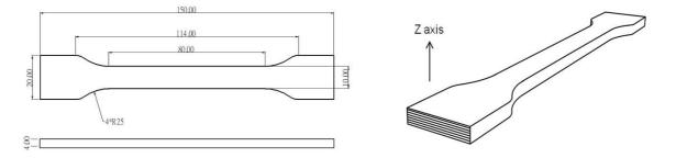
FLEXURAL TESTING SPECIMEN
