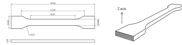
FLEXURAL TESTING SPECIMEN
